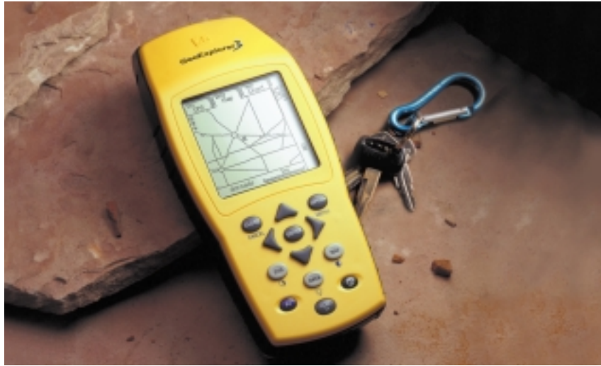
Handheld GPS mapping and GIS data collection/maintenance system.
